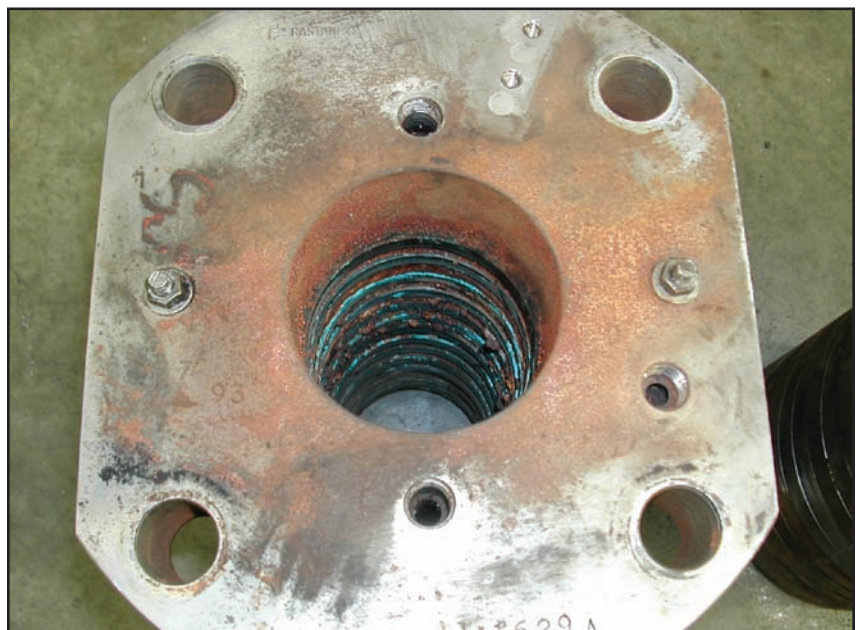
■ Castanet provides a full packing case reconditioning service. After carefully inspecting the worn packing cases, the cups are repaired, finished, ground and lapped. The company follows the same manufacturing process as it uses for new components.
